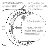
side of the glass cover. Secure the glass cover to lock by pressing the safety pins down and then pushing them one by one under the top screw.
